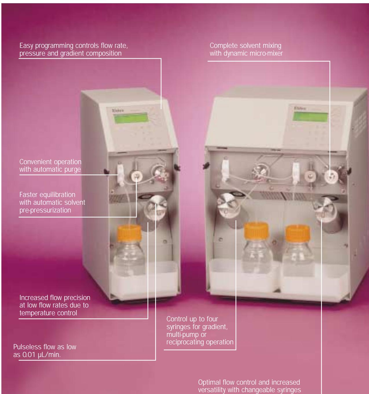
The MicroPro achieves precise, pulseless fluid delivery at flow rates as low as 0.01  $\mu\text{L}/\text{min}$  (gradient flow rates as low as 1  $\mu\text{L}/\text{min}$ ). By taking a system wide approach to developing the MicroPro, we have been able to produce a fully integrated system, in-corporating aspects critical to low flow rate work such as temperature control and minimized system volume.
