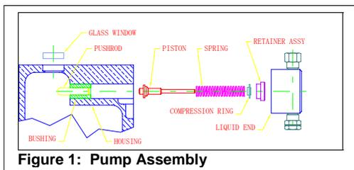
3. Remove liquid end from pump as follows: Unscrew the two socket head bolts (with the 5/32 hex key) while holding the liquid end against the pump housing. Pull the liquid end straight out from the pump housing, in line with the axis of the piston. If you cock or tilt the liquid end, you may break the piston. See Figure 1.
