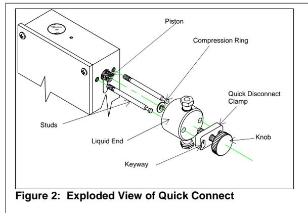
7. Place the quick connect clamp into position on the two studs. The clamp will go over the heads of the studs through the larger hole of the keyway. When the keyway is positioned over the groove (or, smaller diameter) of the stud, slide the clamp down to capture the studs with the smaller hole of the keyway.
